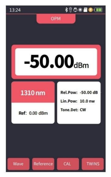
The function is used to test the power of optical signal and insertion loss of various devices and photoelectric components. It can identify and measure the frequency of 270/330/1000/2000Hz optical signal.
