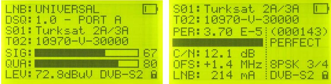
BER / PER : The lower the value of BER in DVB-S1 signals and PER in DVB-S2 signals the better our signal adjustment is.
