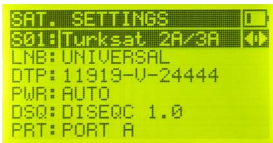
You can make the LNB and Diseqc adjustments of the satellites that are in the memory of the device. These adjustments will allow you to have quick access to commands in the other menus.
