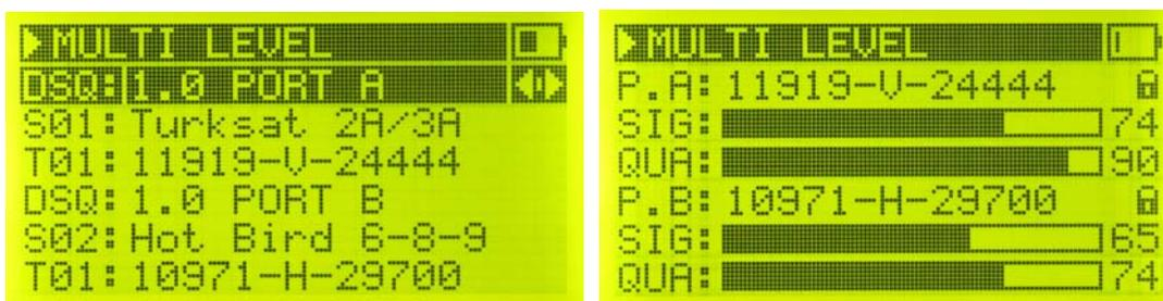
We may see that 2 different satellites in the memory of the device come simultaneously from different Di seqc ports and we may thus make the best adjustment, and we may quickly test the results in the Multiswitch and Di seqc switches, and see the signal and quality details received from the selected TPs.
