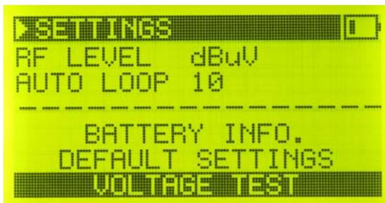
In the SETTINGS menu, you can adjust the Screen Light and the saturation of letters, open and close the Notification sounds, choose among 6 Languages the one that suits you, change the Auto Closing time of your device or turn it off, change the level indicator as dBm or dBuV, and replace the number of satellites in Auto Searches with Auto Cycle numbers.
